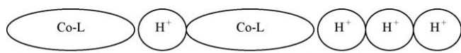
Fig. 8. Monolayer adsorption of cobalt complexes as a result of site competition between hydrogen ions and metal complexes (Co-L: cobalt complex; H + : hydrogen ion).
